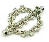
For 2" lines use an 8, 10, or 12mm cable For 3" lines use an 8, 10, or 12mm cable For 4" lines use an 8. 10. or 12mm cable For 6" lines use an 8, 10, or 12mm cable For 8" lines use a 12mm cable
